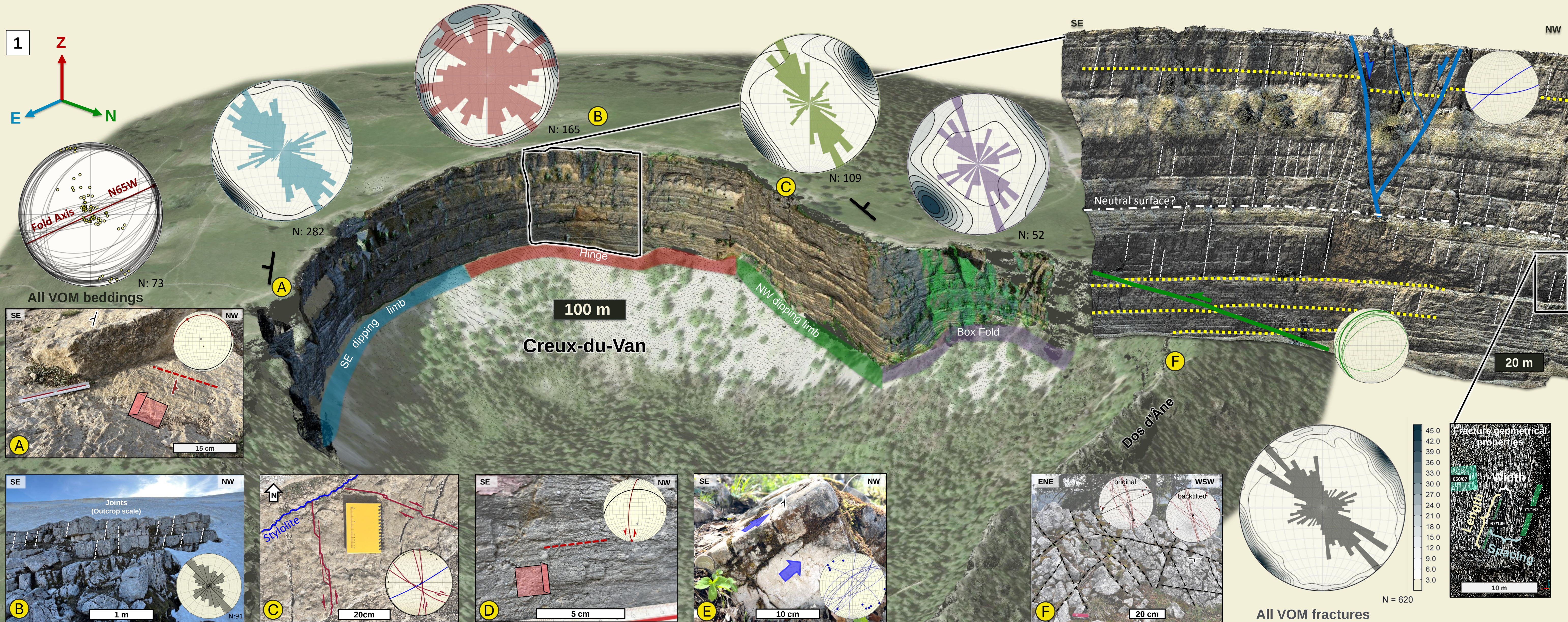
1 – Oblique aerial perspective from the NE showing the terrestrial LiDAR-based Virtual Outcrop Model (VOM) of Creux-du-Van, overlain on the SWISSALTI3D digital elevation model (DEM) point cloud, colored with an aerial photograph [9]. Lower hemisphere equal-area stereograms and rose diagrams represent bedding and fracture orientations from the VOM, interpreted for each sector. Sectors were determined based on their position within a higher-order fold Nouvelle Censière (NC) Anticline (i.e., SE dipping limb, hinge, NW dipping limb, and box fold). A zoomed-in view of the cliff at the Hinge region highlights normal axial faults in the outer arc and thrust faults in the inner arc of the NC Anticline. Another detailed view at meter scale demonstrates how geometrical properties of fractures were measured in this study. Field photographs (A to E) display planar and linear kinematic indicators used in the paleostress analysis, joints were excepted from this analysis, with the associated stereonets showing shear fractures (red), bedding planes (black), and stylolites (blue). Photograph F, taken at the Dos d'Âne, shows steep to vertical bedding and two fracture sets whose intersection is orthogonal to bedding. Note that after back-tilted, the fracture sets appear to form a conjugate set resembling those in image C.
